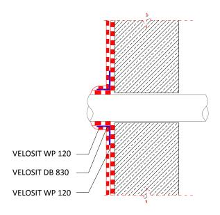
sleeve with a diameter approx. 6 mm (½") smaller than the pipe. The sleeve is made from a 12 cm (5") piece of VELOSIT DB 830. Brush plenty of VELOSIT WP 120, WP 121 or WP 124 onto the pipe and the surrounding area. Pull the sleeve over the pipe push it with a trowel into the material. Work away from the pipe and take care not to entrap air or create wrinkles.
